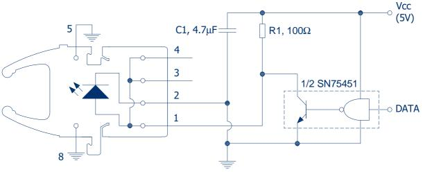
FIGURE 2 Recommended transmitter application circuit. See note 4 Table 6
