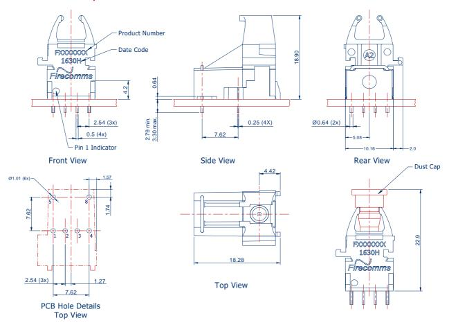
FIGURE 7 Mechanical dimensions of the vertical receivers and PCB footprint, which is a top view. General dimensional tolerance is  $\pm\,0.2$  mm
