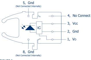
FIGURE 1 Receiver pin-out, top view.
