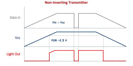
FIGURE 10 FE50MLNR Non-Inverting Tx operation during power cycling with input logic high
