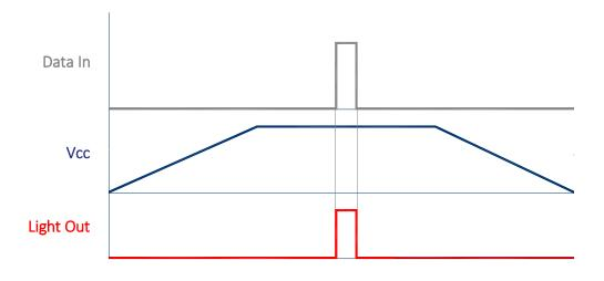
FIGURE 6 FE50MLIR Non-Inverting Tx operation during power cycling with input logic low
