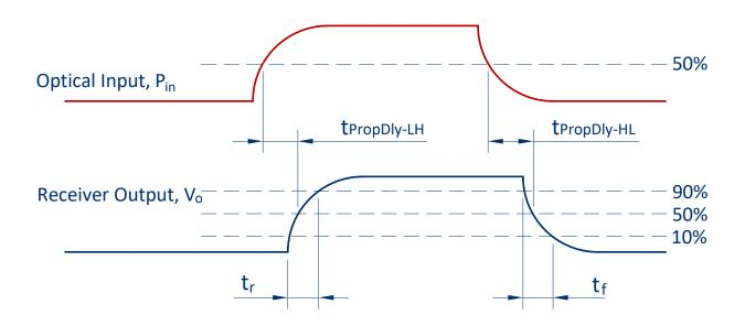
FIGURE 9 FE50MLNR Receiver Propagation Delay and rise/fall time definitions for a non-inverting  $V_0$  output
