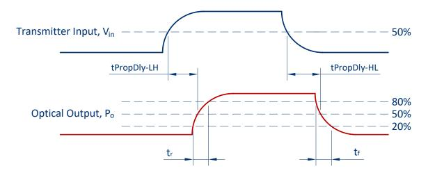
FIGURE 3 FE50MLIR Transmitter Propagation Delay and rise/fall time definitions
