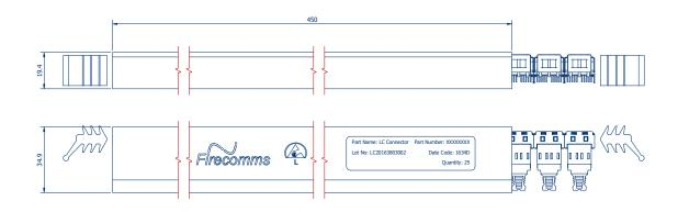
FIGURE 14 Packing tube for Firecomms FE50MLIR FE50MLNR LC Transceivers
