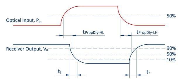
FIGURE 4 FE50MLIR Receiver Propagation Delay and rise/fall time definitions
