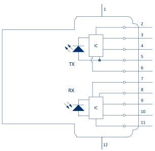
FIGURE 1 Transceiver pin-out, top view
