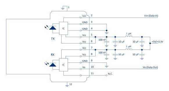
FIGURE 2 Recommended application circuit
