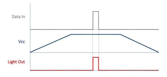
FIGURE 11 FE50MLNR Non-Inverting Tx operation during power cycling with input logic low
