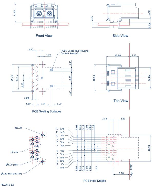
Mechanical dimensions of the product, and PCB footprint, which is a top view General dimensional tolerance is  $\pm$  0.2 mm
