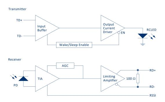
FIGURE 3 Electronic block diagrams of the transmitter and receiver fiber optic transceivers
