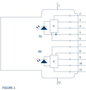
Transceiver pin-out, top view
