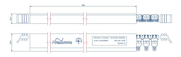
FIGURE 10 Packing tube for Firecomms LC Transceivers
