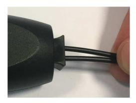
(6) Connect the CAT5 cable to both the media converter and the target equipment (e.g. a laptop, desktop, set-top-box or router).
